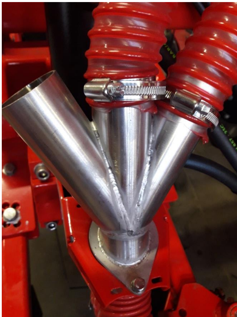
Fig. 65. Connecting the fertilizer hoses to the distributor of the working section
