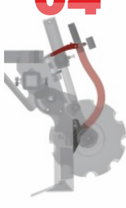
NOZZLE FOR FERTILIZER APPLICATION Ensure precise application of one or two types offertilizer along the soil profile
